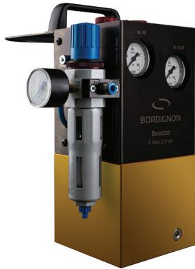
The Bordignon Booster is a pneumatic pump. By using compressed air, it increases the nitrogen N<sub>2</sub> pressure during the charging operation of gas springs for dies, in a safe and very precise way. Light and compact, the Bordignon Booster has a low compressed air consumption, resulting in savings of time and costs.
