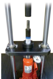
This device is a load gauge for nitrogen gas springs. This device is usually used to measure the initial force of nitrogen gas springs, in order to verify that they are actually charged.
