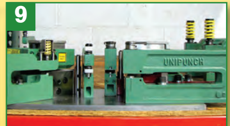
The tooling in the dedicated setup is assigned to the part for the life of the part. Here it is shown stored on a shelf, ready for the next time that part is required.
