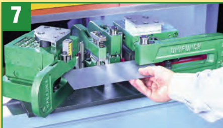
Depending on the application, material can be hand fed (as shown) or fed off a coil.
