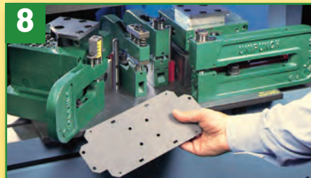
You can punch and notch multiple holes with each stroke of the press.
