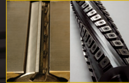
CUTTERHEAD OPTIONS Available with 40 four-sided carbide inserts for the helical cutterhead or a 3-blade, high-speed steel straight knife cutterhead
